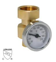
Caleffi 521 and 5231 series mixing valves are available with optional outlet temperature gauge, or field installed with point of distribution low-lead brass mixed temperature gauge adapter (above) replacing the existing threaded union outlet nut and tailpiece. Removable 2" gauge fits into temperature well.
