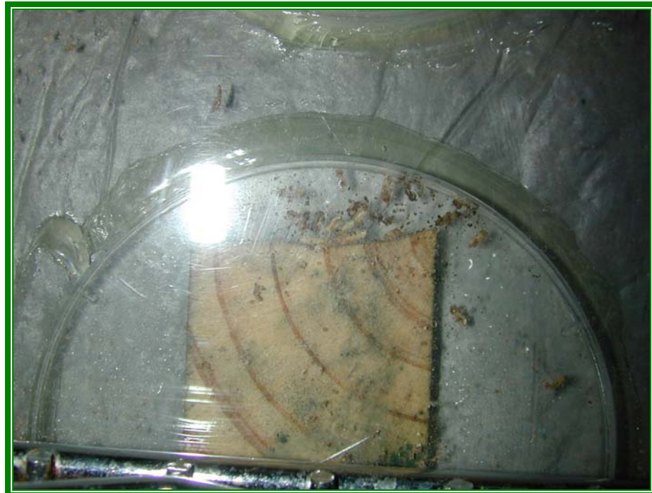
Termite penetration through Sopraseal LM 200 T (Underside View)
