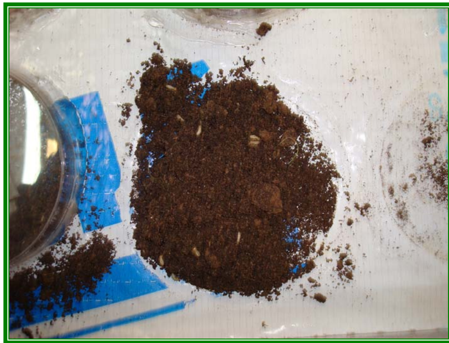
Termites over Colphene ICF
